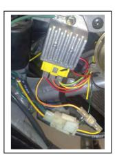
7. →IMPORTANT: protect the other end of the yellow electrical system wire previously cut with insulating tape.
