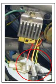
4. →Connect the female terminals to the male terminals of the regulator connector in the order given in the layout.
